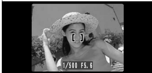
When you press the shutter button down halfway, the camera emits a short double-beep and focuses on your subject (the viewfinder lamp (green) changes from blinking to steady). At that point, the AF frame on the LCD monitor becomes smaller and the camera sets the shutter speed and aperture.
