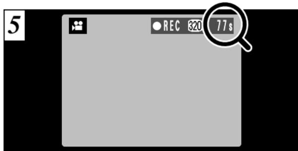
During shooting, a timer in the top-right corner of the LCD monitor counts down the remaining time.
