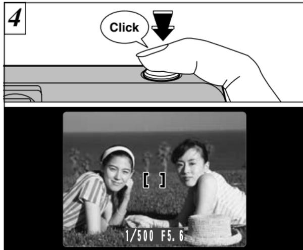
Continue to hold the shutter button down halfway. Move the camera back to the original image and then fully press down on the shutter button.
